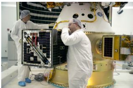
AeroAstro engineers integrate STPSat-1 onto the ESPA ring.
